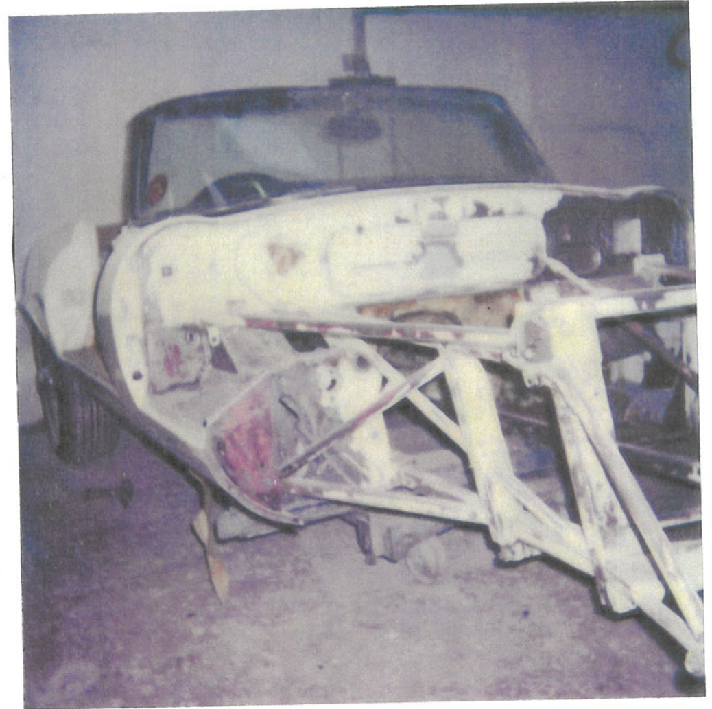
Photographs 9 and 10 – Chassi almost and completely stripped, hoisted for any repairs
